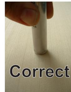
MAG-ic Probe is capable of measuring very small distances to 1/1000th inch. It should make sense then that the probe should be absolutely square to the surface being measured and the opposing magnet. If the probe is slightly tilted, the distance from the center of the probe will be slightly farther from the magnet and introduce false readings. It is a good idea to use the **HOLD** mode to ensure the lowest reading by making small rocking and circling motions at each measuring location.
